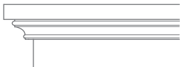
Top with Trim EST-CH Adds 1" to overall height. Adds 2" to overall width.
