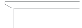
Top with Reverse Bevel EST-RB Adds 1" to overall height. Adds 2" to overall width.
