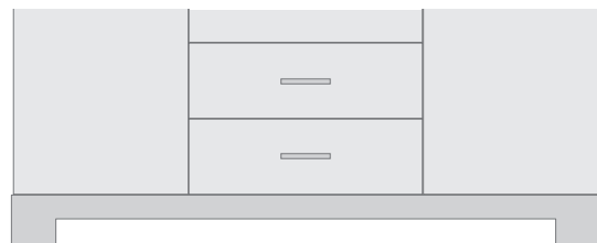
Cutout Base ESFUL-L-CO, Adds 4" to overall height.
