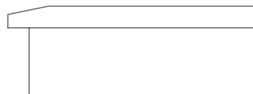
Top with Large Bevel EST-LB Adds 1" to overall height. Adds 1½" to overall width.
